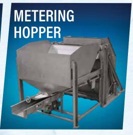
Hoppers for bulk loading while regulating the discharge of product by using an adjustable slide gate and vibratory conveyor.
